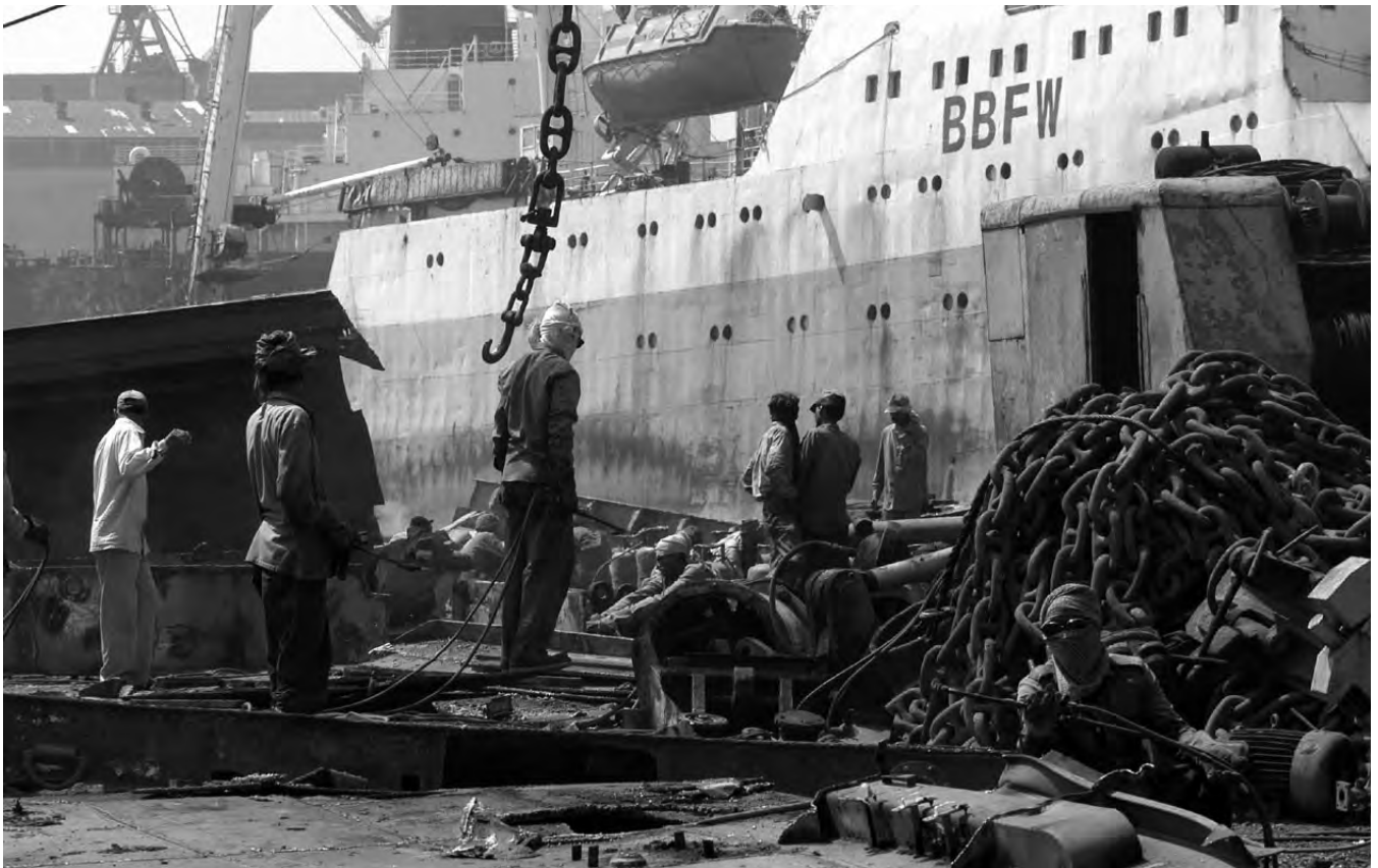
Shipbreaking in Mumbai. Worker with blowtorch, termed the "gas cutter." Workers prepare to walk metal girder further up the beach for cutting.
