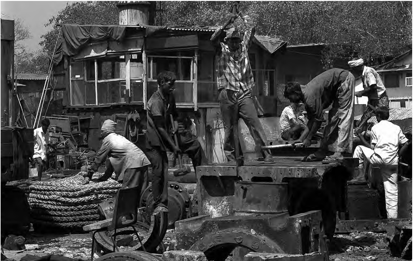
Shipbreak in Mumbai. Men wielding sledgehammers break up heavy marine engines for salvage. Heavy marine diesel engines are repaired, broken, or cannibalized.
