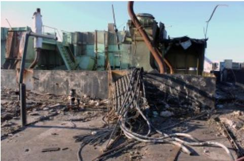
The "Tellier" had just been stripped of 50 tons of asbestos and was still lying in water. According to Peter Wyntin, the company's Head of shiprecycling, Environment Manager and Health & Safety Manager, the several months it took to remove all the friable and non-friable asbestos onboard represented the most expensive recycling phase. As it was common to use asbestos in ships for almost any type of application, from glue to insulation, it can be found practically anywhere
